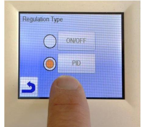
9) If you wish to use PID mode select "PID" red dot should be lit as in above picture otherwise return to main screen by pressing the return
