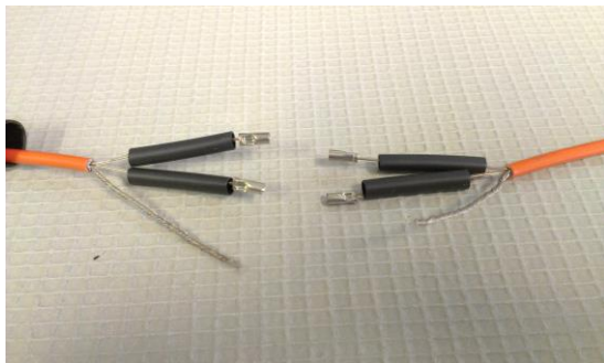
11) Slide a black sleeve over each butt connector.
