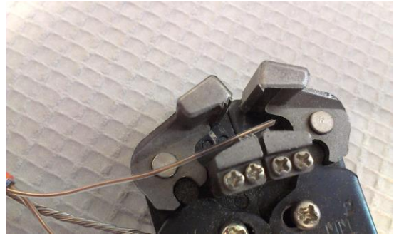
8) Strip 5mm off each power wire.
