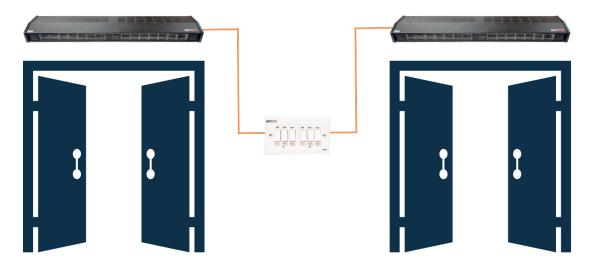
The new CS-9 switch is ideal for controlling two overdoor heaters in a commercial application
