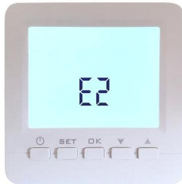
E1 or E2 fault codes are displayed if the temperature sensors are faulty or are not connected. The thermostat will stop heating until the fault is corrected.
